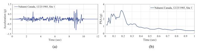
Figure 6. The 1985 Nahanni earthquake: (a) recorded acceleration, (b) pseudo spectral acceleration.
