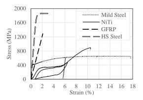
Figure 2. Stress-strain relationships of reinforcing materials.
