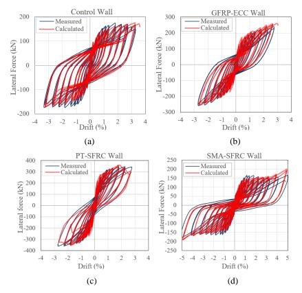
Figure 5. Calculated and measured hysteretic responses specimens: (a) CW, (b) GFRP-ECC, (c) PT-SFRC, (d) SMA-SFRC.
